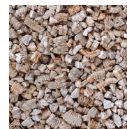
vermiculite attic insulation
