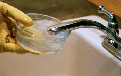
Soaking the tap with the bleach solution
