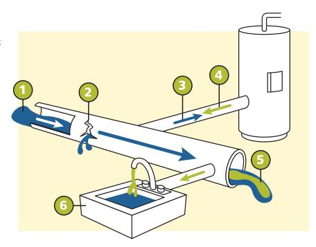
Providing an air gap between the water supply outlet and the flood level rim of a plumbing fixture or equipment prevents contamination that may be caused by backflow.
