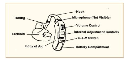
hook, earmold, volume control, on/off switch, and battery compartment.
